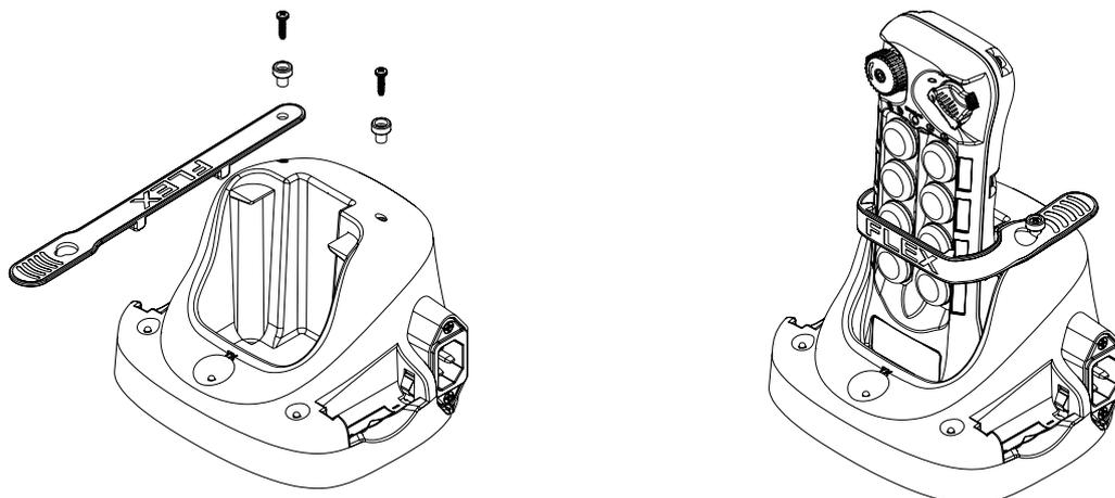
3) If mounting bracket is used (optional), slide down the charging station along the guided track to secure the charging station to the mounting bracket. Remove the charging station by pressing down the bracket release and pull the charging station upward until it clears the guided track.
